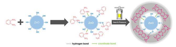
Figure 1. Synthetic process of the ZnO@C NPs
