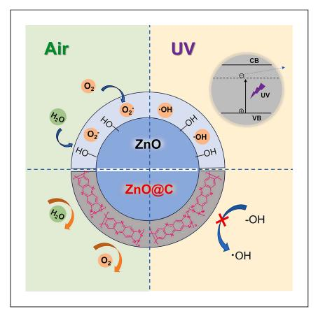
High UV and air stability are critical for the future application of organic solar cells (OSCs) in architectural integration and outer space. Yan et al. report carboncoated zinc oxide as electron transporting layers for OSCs, which can significantly improve both their power conversion efficiency and air/UV stability. Lingpeng Yan, Yu Wang, Wensheng Zhao, ..., Qingmei Su, Hua Wang, Chang-Qi Ma
